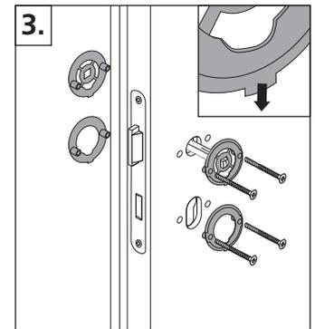
4. Break inner plastic part on the pre-defined breaking areas and remove.
