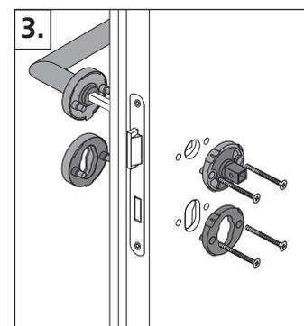
4. **! Attention !** The spindle must protrude at least 5 mm from the anchor to ensure perfect handle guidance!
